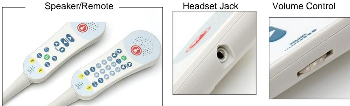
To use the headset, simply plug it into the side of your speaker/control device. Put the headset over your head, locate the ear pads on your ears, and adjust the volume to a level that is comfortable for you.
